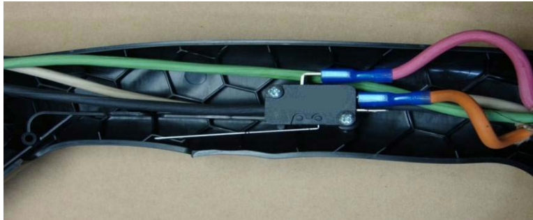
Fig.6-4 Switch Wire Location
