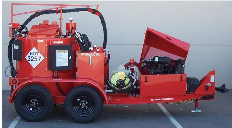
Super Shot 125 Diesel Melter with Air Compressor 70CFM PN 45500
